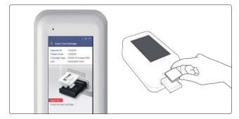
Prepare a test sample and inject it (either 1-2 drops with reagent tube or 50µL with pipette) according to the Sampinute<sup>™</sup> Analyzer User Manual. Touch 'OK' to initiate analysis.
