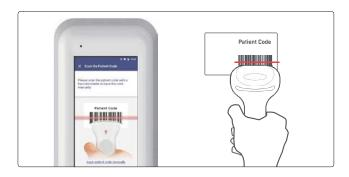
4. Scan QR code on cartridge pouch with barcode scanner. Open pouch to take out test cartridge.
