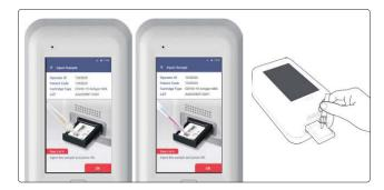
7. When the test is completed, the results are displayed on the touch-screen.
